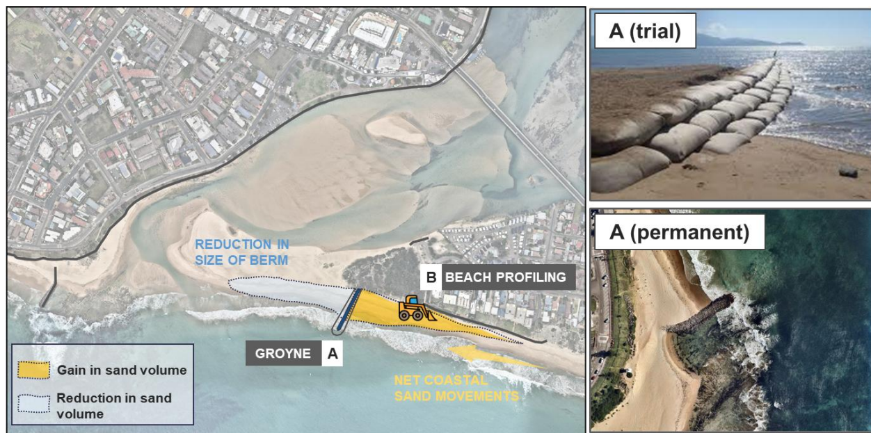
Figure 74: Northern groyne (Option B2) conceptual design layout.
