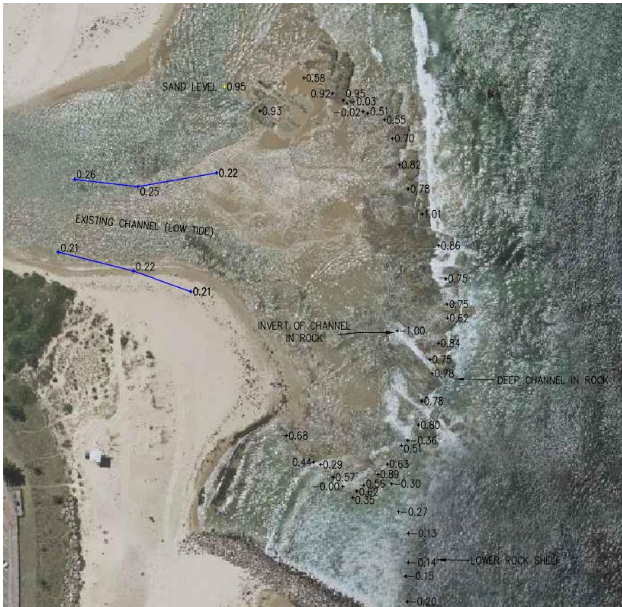
Figure 11: Rock shelf survey undertaken by CCC in 2020 (Glamore et al., 2021).
