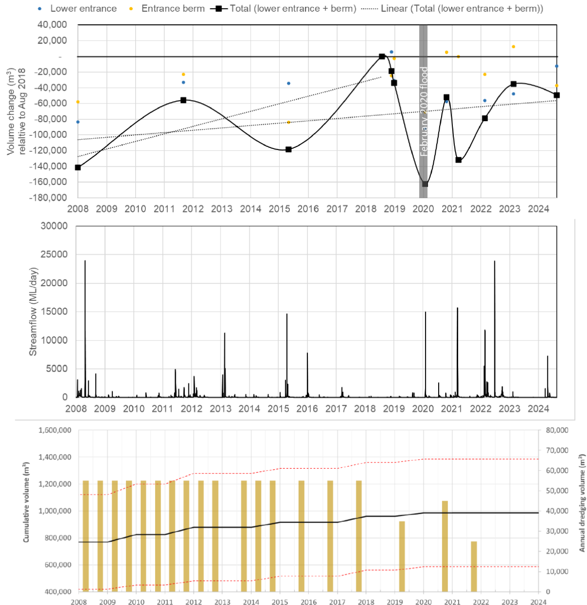
Figure 43: (top) timeseries of sand volume changes in the entrance area, (centre) Wyong River stream flow and (bottom) entrance dredging activity.
