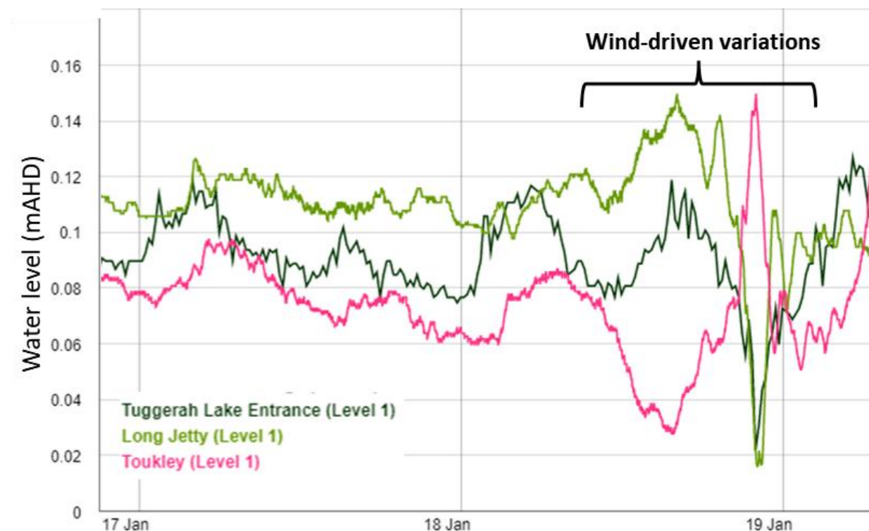
Figure 23: Seicheing observed in water level gauges at opposite ends of Tuggerah Lake during strong wind event in January 2023.
