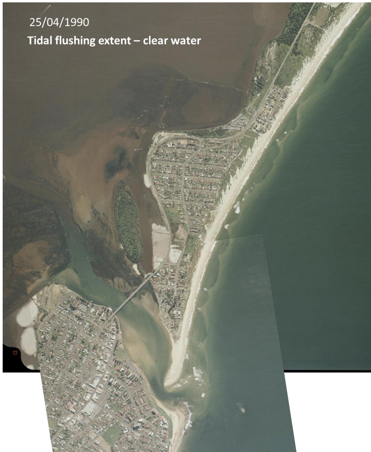
Figure 35: Example aerial photograph captured 25 April 1990 showing spatial extent of tidal flushing (clear water) at Tuggerah Lakes entrance following high catchment runoff (source: NSW Government). At the time of this photo reclamation activities are underway and Terilbah Channel is blocked.
